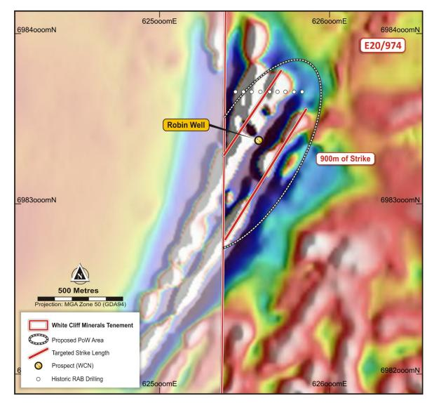
*Figure 6:* Robin Well prospect over magnetics, highlighting the targeted strike length to be tested by first pass soil sampling
