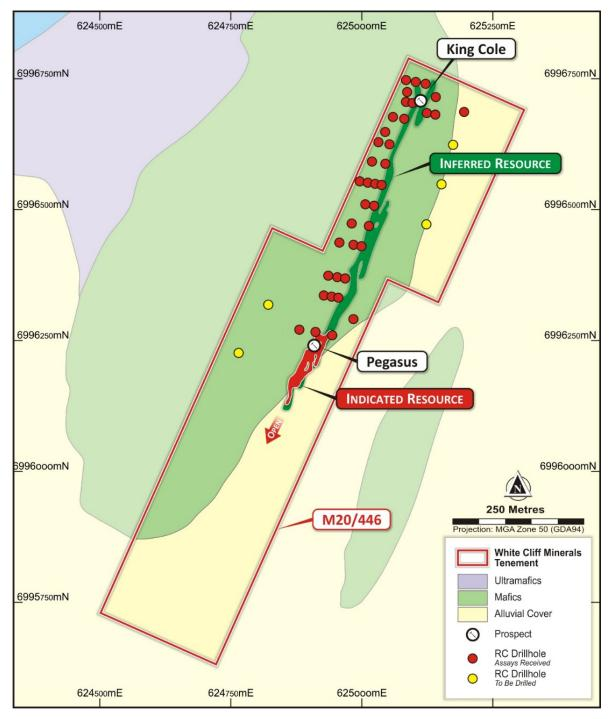
Figure 1: Location of RC drilling program at the Reedy South Gold Project
