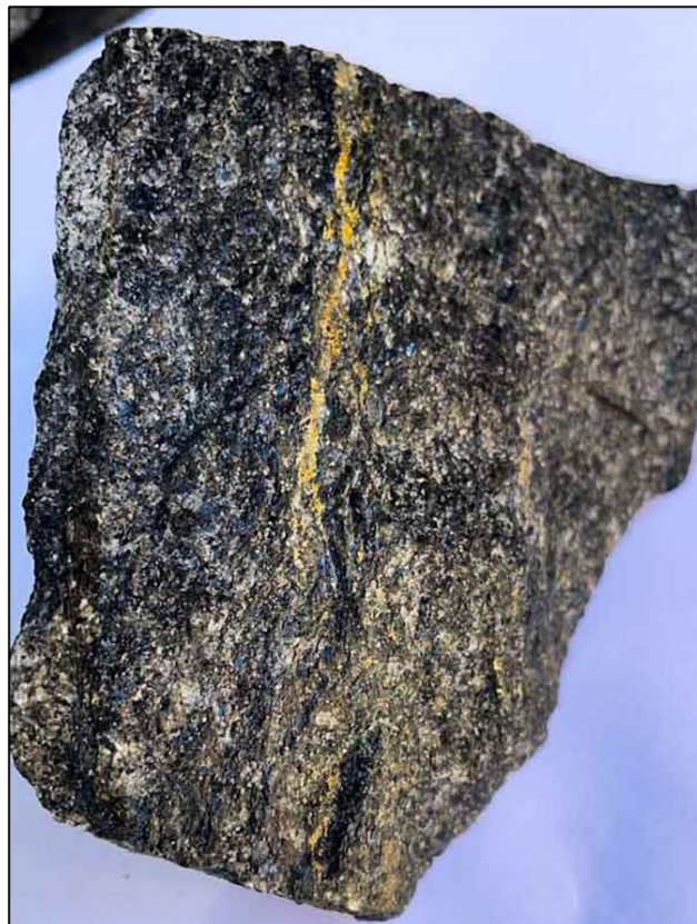
Figure 1. Chalcopyrite veinlets and chalcopyrite + pyrite ± bornite matrix mineralisation in silicified Amphibolite (15cm)
