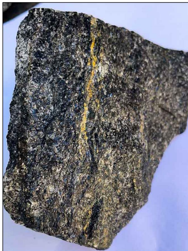
Figure 1. Chalcopyrite veinlets and chalcopyrite + pyrite ± bornite matrix mineralisation in silicified Amphibolite (15cm) (Sample 1)
