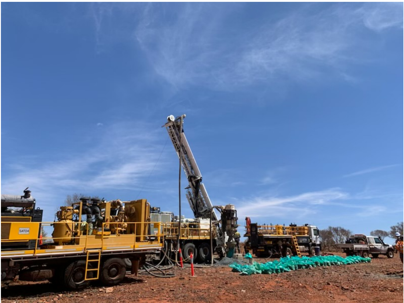
Figure 3: RC drill rig in operation at Stakewell
