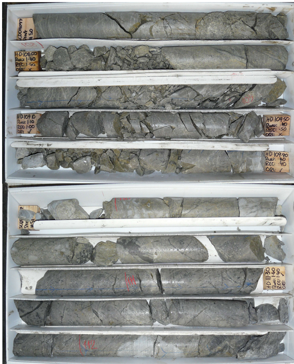
Figure 3: Mineralised drill core from diamond drill hole SCDDH097 (107.4-112.4m) at Sams Creek showing silicified and altered dyke with dark grey sulphide veins dominated by arsenopyrite
