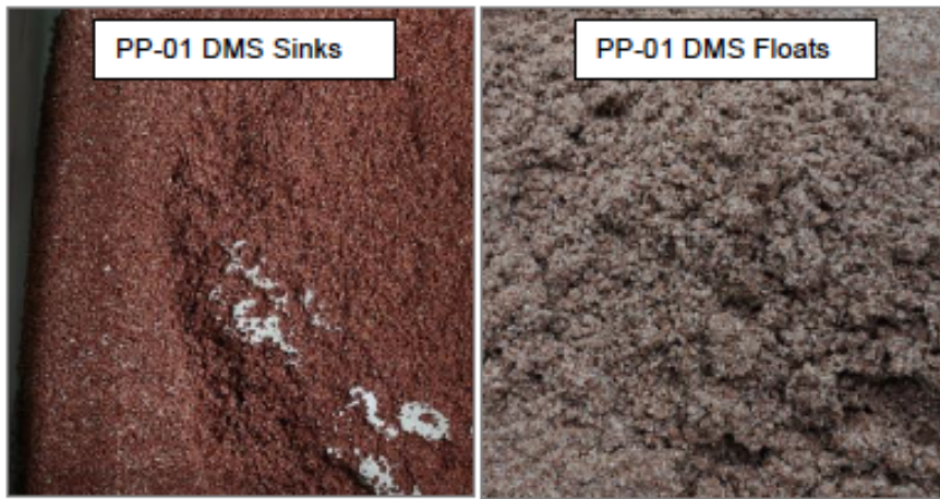
Figure 6: DMS separated products featuring Sinks containing high grade bastnaesite product (red) and Floats containing non-mineralised material
