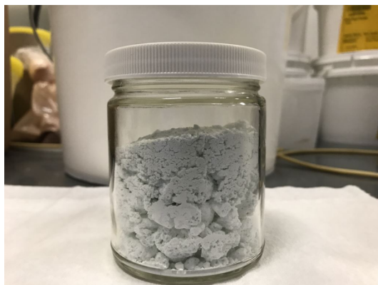
Figure 1: Mixed rare earth carbonate produced to target impurity levels
