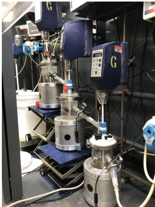
Figure 10: Leaching and Precipitation equipment prior to the commencement of the bulk carbonate production program
