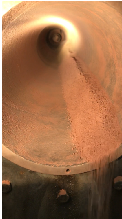
Figure 9: Kiln operations showing free-flowing beneficiated product exiting the kiln in preparation for the commencement of the leaching program
