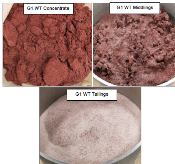
Figure 8: Wilfley Table beneficiated products after a single pass (-0.5+0.25mm size fraction). WT Concentrate and Middlings were combined to produce feed for the leaching program
