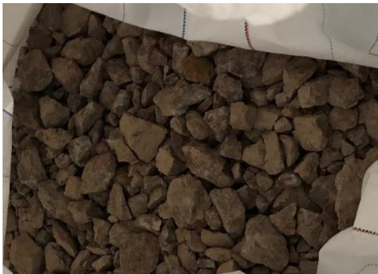
Figure 4: Beneficiated product following ore sorting
