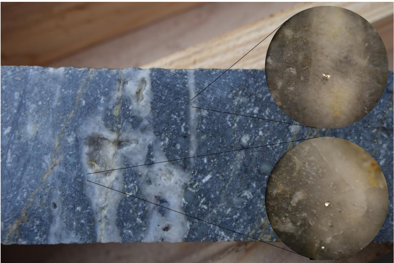
Figure 1: Visible gold associated with pyrite in drusy, fine grained, white chalcedonic quartz at 68.8m in UGA-07
