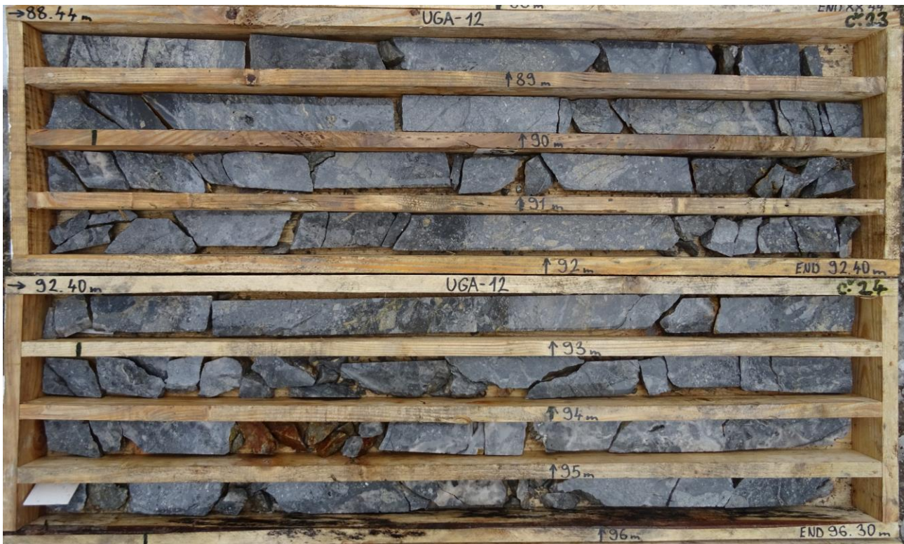
Figure 4: UGA-12 drill core; interval from 17m to 102m (down-hole) showing quartz filled vein/stockwork/breccia structures, variably rich in fine to very fine grained sulphides (mainly pyrite/marcasite) and hosted within strongly argillic altered andesite host rock. Traces of visible gold identified at 95.1m to 95.2m
