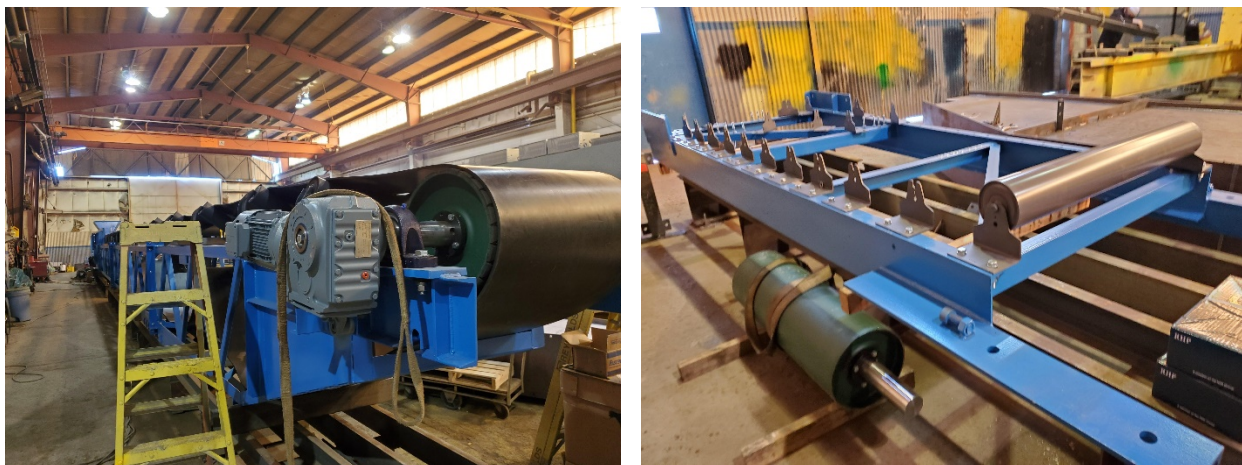
Figures 3 and 4: Feed conveyor and belt feeder for Vital Metal's ore sorter at Nechalacho
