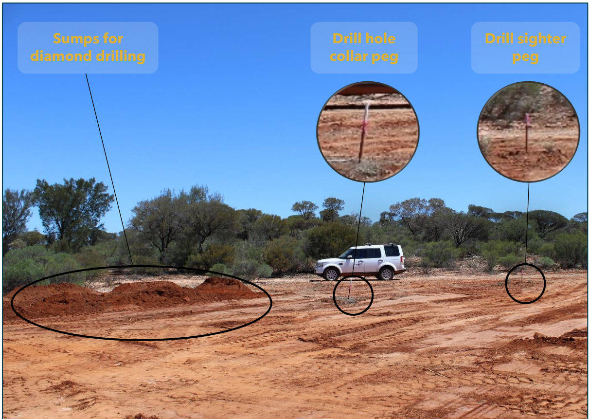
Figure 2: Drill pad for hole VDD011 cleared ready for drilling.
