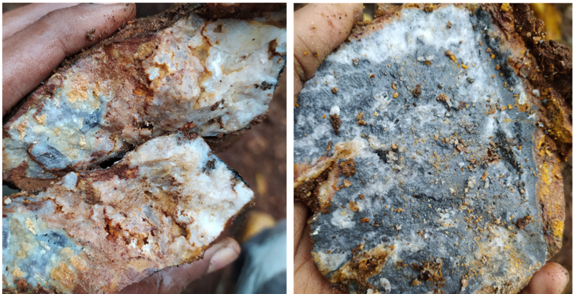
Photo 4: Quartz (left) and quartz-sulfide (right) veins (OC) at 17 m interval of KC24.
