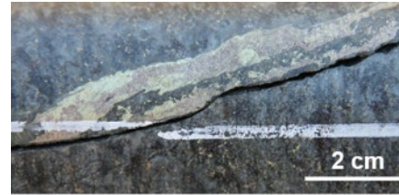
Late – stage pyrrhotite – chalcopyrite vein set with disseminated sulphide at 121.6m @ 121.6m
