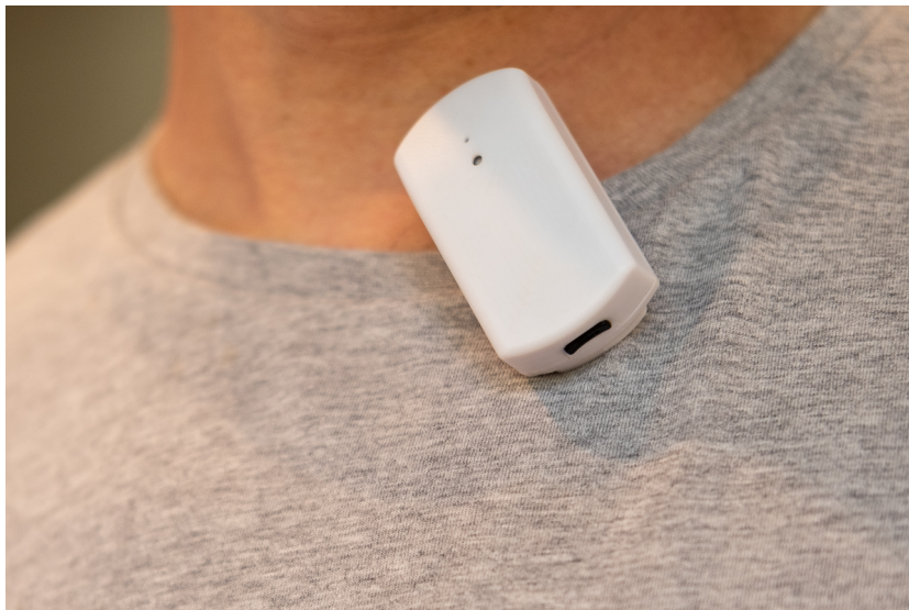
Image Two: ResApp's wearable device is an easily worn, clip-on, unobtrusive platform, which allows for continuous patient monitoring using cough audio.
