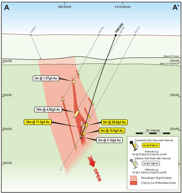
Figure 2: Hercules prospect cross-section A-A', central area, note multiple lodes in TNRC020.
