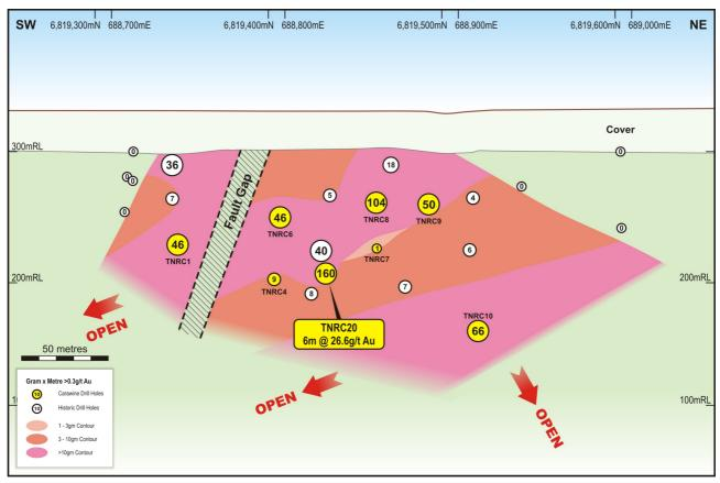
Figure 1: Hercules prospect long section along the main mineralised zone. The circle labels are of gram-metre intervals for the reported results from Carawine's drill holes (yellow) and historic results (white).
