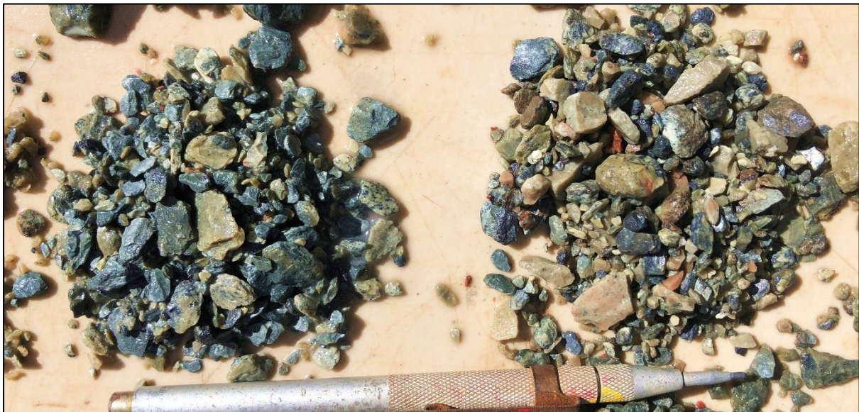
Figure 2: RC chips from hole AC3RC004 mineralised interval 89-91m. The grey mineral is galena (lead sulphide), red mineral is sphalerite (zinc sulphide).
