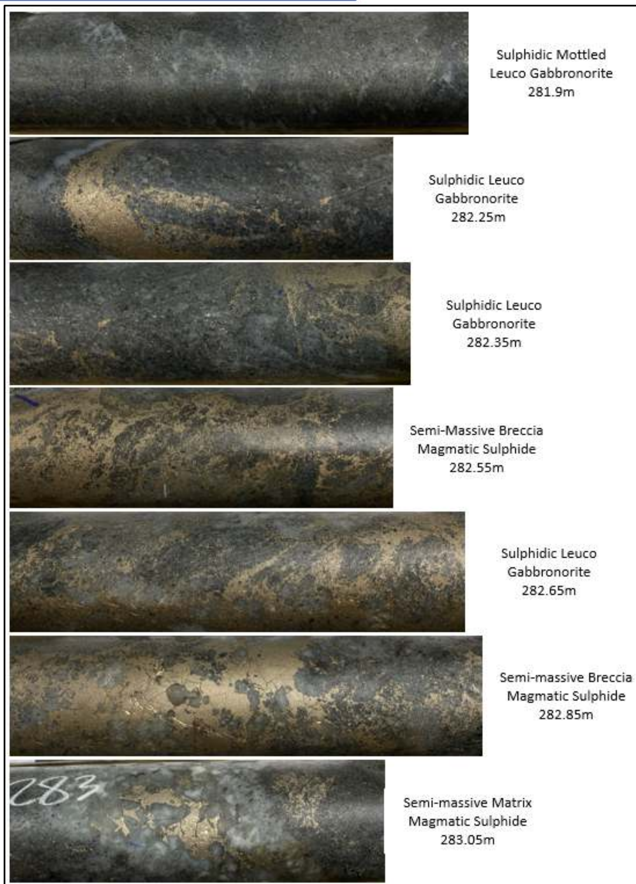
Figure 2 – Core photos of sulphide zone at about 282m downhole
