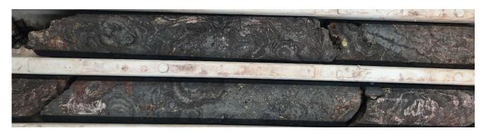
Figure 3: VUD018, colloform massive hematite breccia at ~1387m, NQ core.
