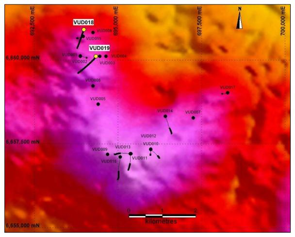
Figure 2: Vulcan Prospect, residual gravity image showing location of VUD 18 & 19 and previous Tasman drill holes. The thick black lines on the drill hole traces are the surface projections of basement intercepts (Grid GDA 94, Z53).
