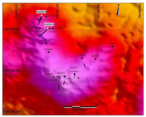
Figure 2: Vulcan Prospect, residual gravity image showing location of VUD 0018 & 0019 and previous Tasman drill holes. The thick black lines on the drill hole traces are the surface projections of basement intercepts (Grid GDA 94, Z53).
