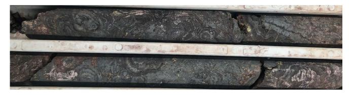
Figure 3: VUD0018, colloform massive hematite breccia at ~1387m, NQ core.
