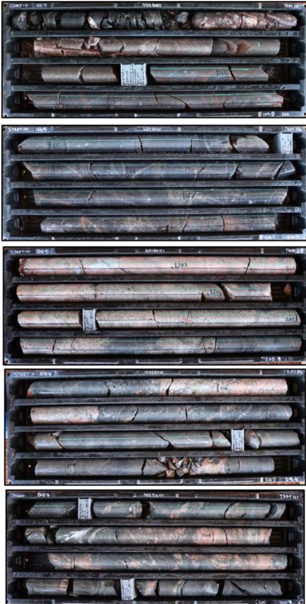
Figure 4: Selection of core tray photos of hole NDIBY01 as published by GA. Core depths are shown on each tray.
