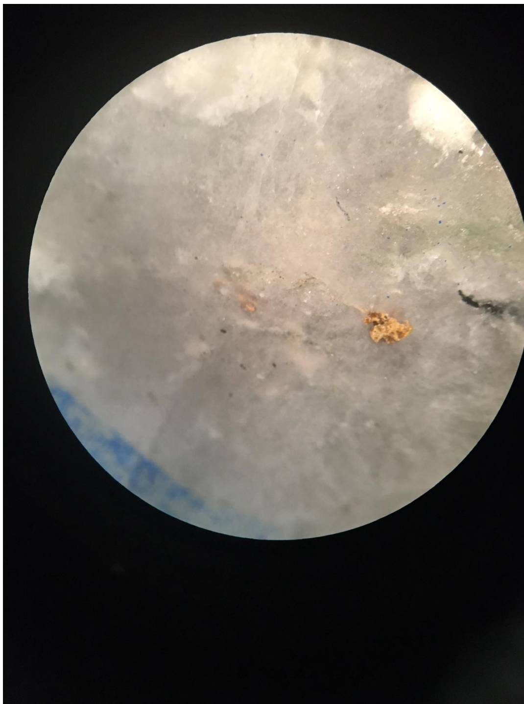
Plate 4: Visible Gold in quartz in diamond drill hole FEDD052 at 338 metres at Boyd North. Field of view 4mm.
