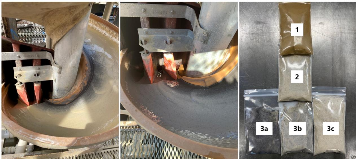
Figure 3: Spiral testwork and heavy mineral concentrates at the Mineral Technologies lab in Starke, FL (Sample 1. Ore, Sample 2. Deslimed Ore, Sample 3.a. Concentrate, Sample 3.b. Middlings, Sample 3.c. Tailings).
