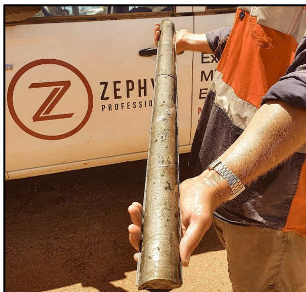
Figure 3: Photo of massive nickel sulphide in drill core of diamond hole TED07 at the Dusty nickel discovery on Toro's 100% owned Yandal Gold Project – this part of the core grades 4.01% nickel (see text for details).
