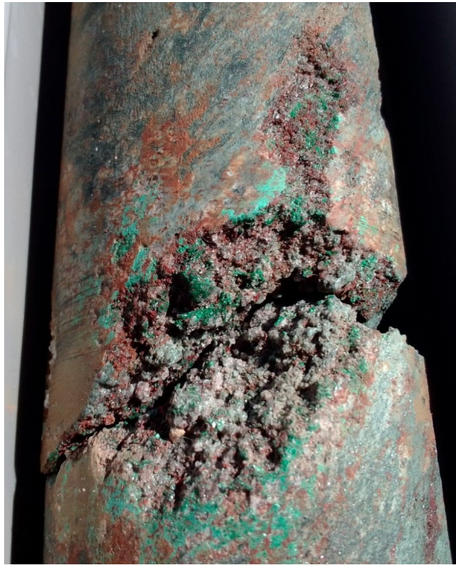
Figure 2 – Photo of Malachite mineralisation within HQ3 Drill Core at approximately 317.8m with drill hole FPDD003. Width of HQ3 drill core – 61.1mm
