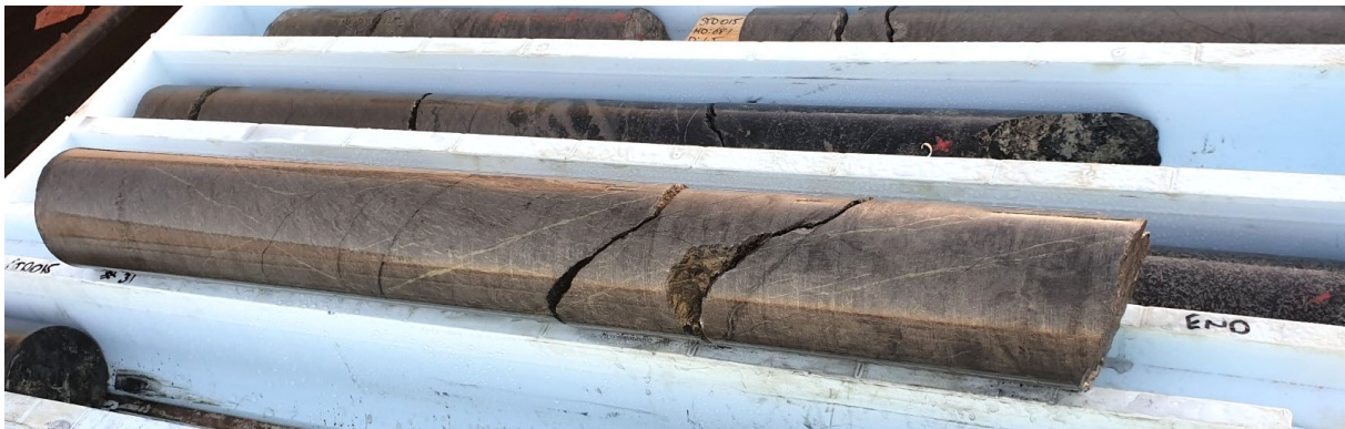
Figure 4 – drill core tray for STD015 – one of the additional metallurgical holes completed at Stricklands – showing massive sulphides intersected from 67.3m downhole.
