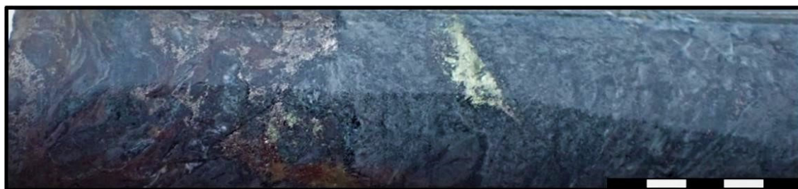
Picture 2: Drill core from KI0DD002 (92.7m) – blebs of pyrrhotite-sphalerite-chalcopryrite hosted in quartz-chlorite-actinolite altered volcanic siltstone
