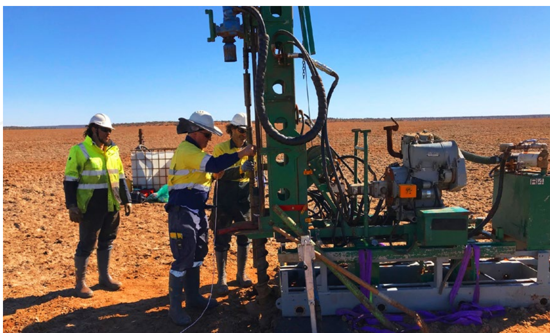
FIGURE 4: LAKE THROSSELL HELICOPTER SUPPORTED ROTARY DRILL RIG.
