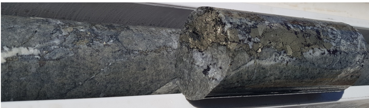
Figure 3. Strongly mineralised drill core from BCDD372, 150m down hole & 40m along strike from the open pit
