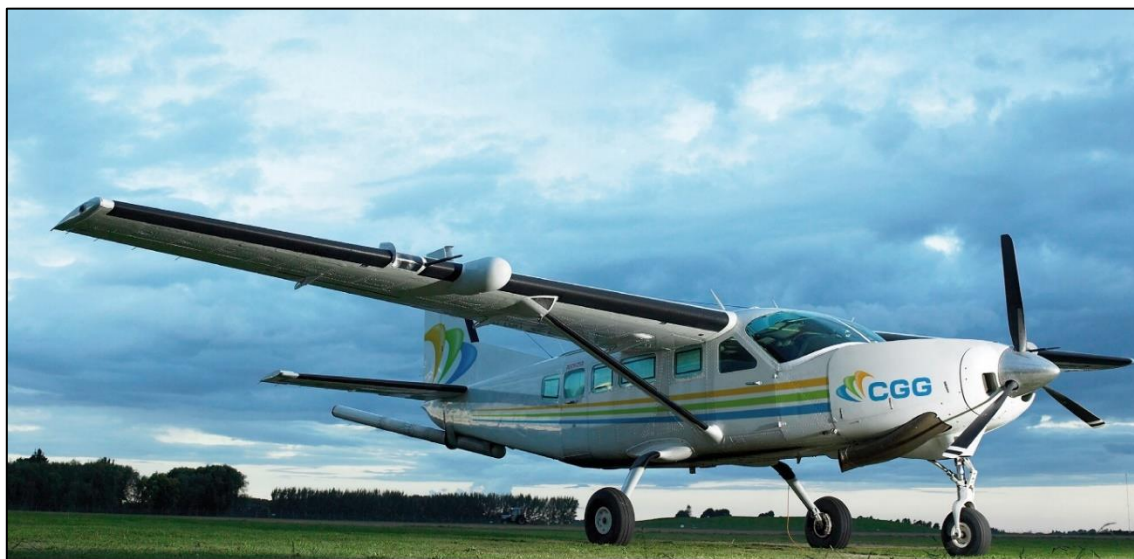
Figure 5. The Cessna Caravan Falcon™ gravity gradiometer survey plane.
