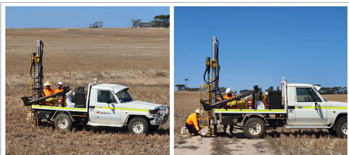
Fig 2 – Sahara Operations Pty Ltd auger rig and field crew conducting sampling at the Viper Project
