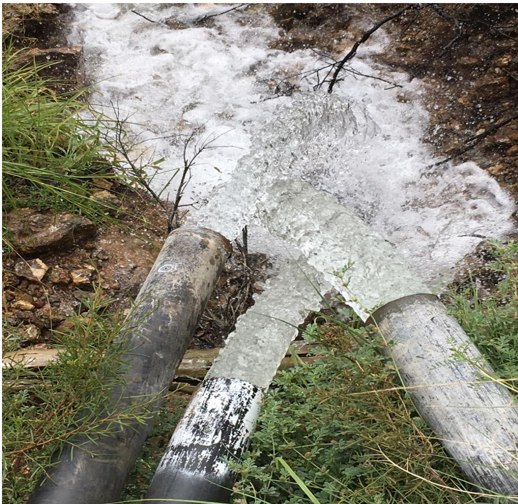
Figure 13: Dewatering bores into evaporation ponds at Mt Freda open cut to 200m.
