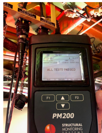
Figure 2: PM200 Test box indicating SLS Lead 6 (zone with approximately 30 fasteners) Passed.
