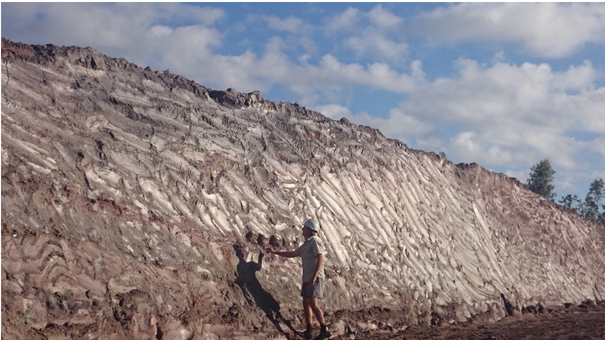
Figure 3: Mining of soft, weathered, graphite rich regolith at the Graphmada Mine.
