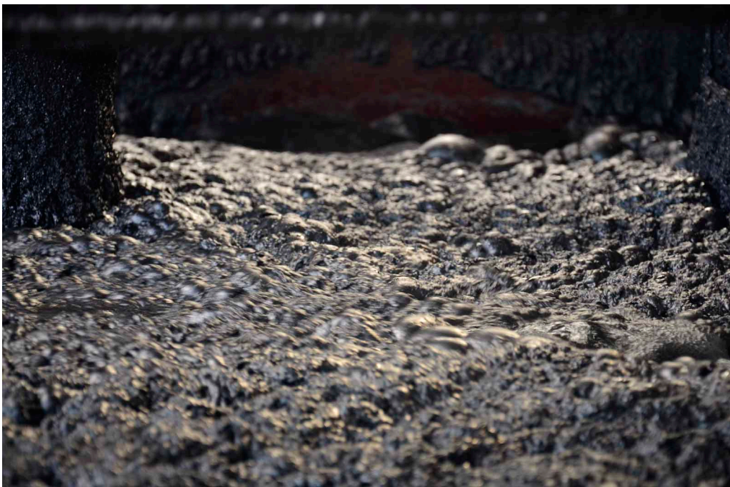
Figure 5: Flotation of large flake graphite for analysis.
