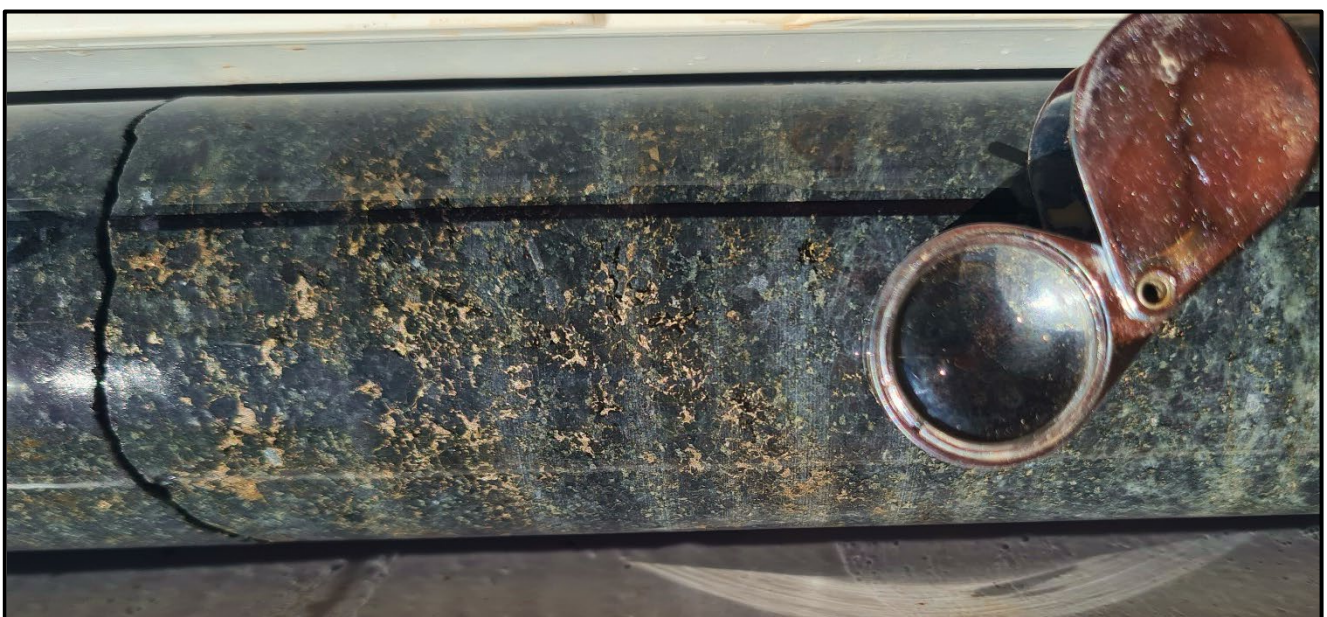
Figure 1 — Disseminated Sulphide in LADD003 at 170m (pyrrhotite with minor pentlandite/chalcopyrite)
