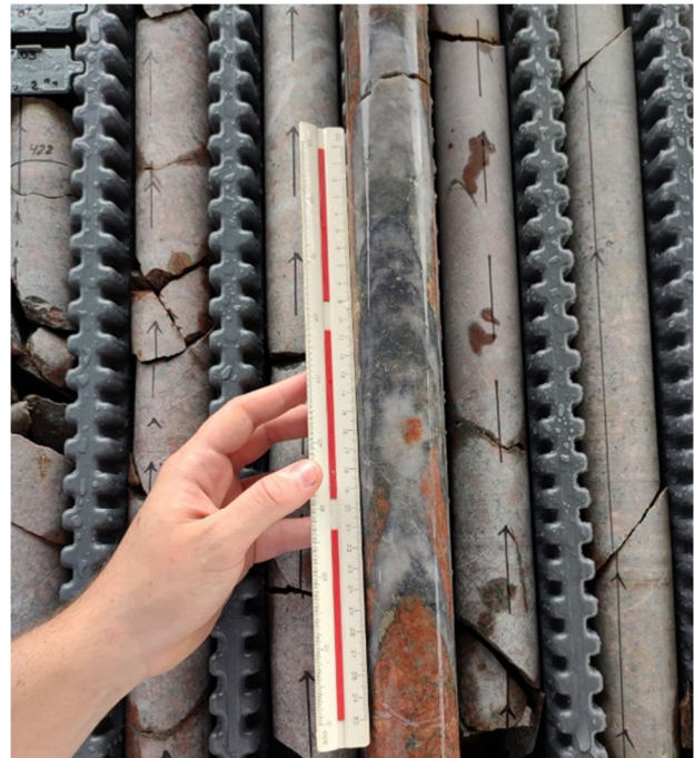
Photo 04: Quartz vein with pyrite (Py) and molybdenite (Mo) intercepted at 444m downhole.
