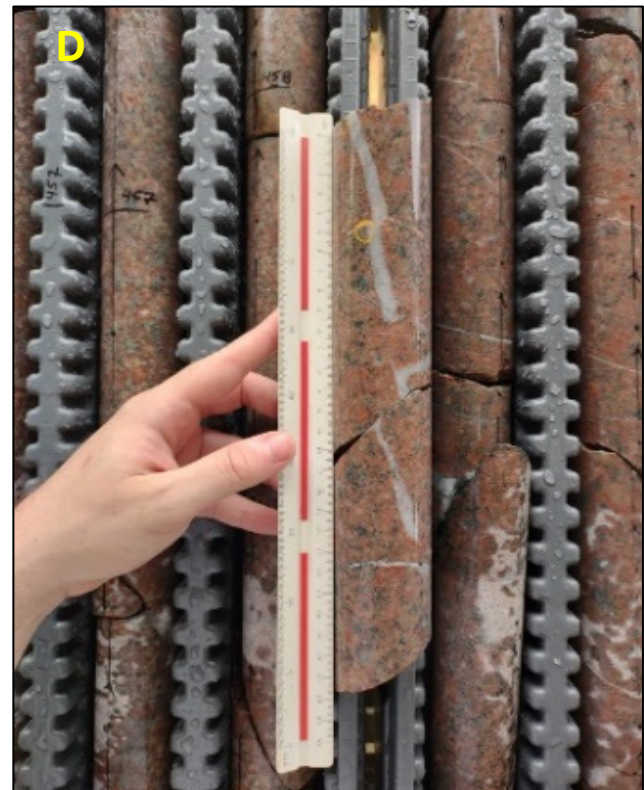
Photo 05 – a and b) M Type veinlets (magnetite in quartz) in the porphyritic granite (GRpf) with propylitic alteration (PR1) and; c and d) B type veins with molybdenum in the GRpf with PR1 alteration.
