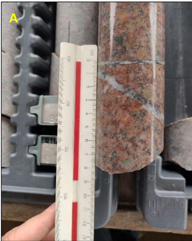
Photo 05 – a and b) M Type veinlets (magnetite in quartz) in the porphyritic granite (GRpf) with propylitic alteration (PR1) and; c and d) B type veins with molybdenum in the GRpf with PR1 alteration.
