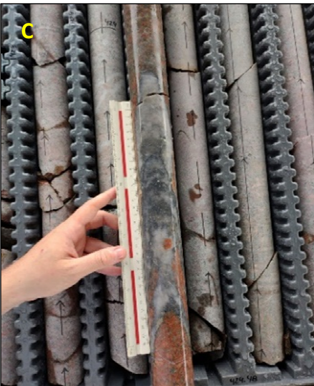
Photo 05 – a and b) M Type veinlets (magnetite in quartz) in the porphyritic granite (GRpf) with propylitic alteration (PR1) and; c and d) B type veins with molybdenum in the GRpf with PR1 alteration.
