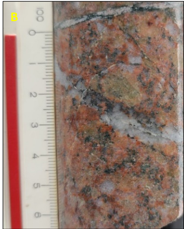
Photo 05 – a and b) M Type veinlets (magnetite in quartz) in the porphyritic granite (GRpf) with propylitic alteration (PR1) and; c and d) B type veins with molybdenum in the GRpf with PR1 alteration.
