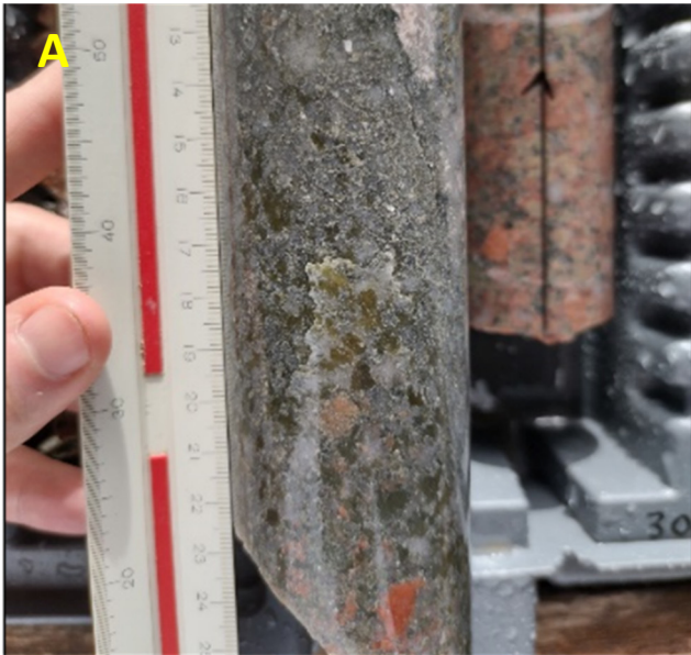
Photo 03:- a) Quartz-Pyrite veinlet (VQP) and b) Coarse phengite haloes to the VQP.
