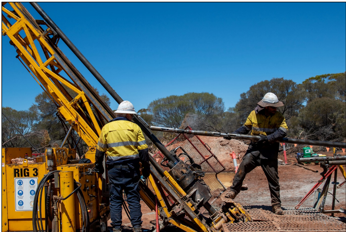
Figure 4; Inner tube being retrieved from hole VDD001
