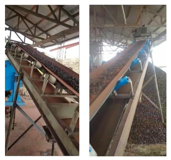
Figure 4: Crushing and screening of Apurimac ore underway at local plant to produce high grade Apurimac Premium Lump DSO product.
