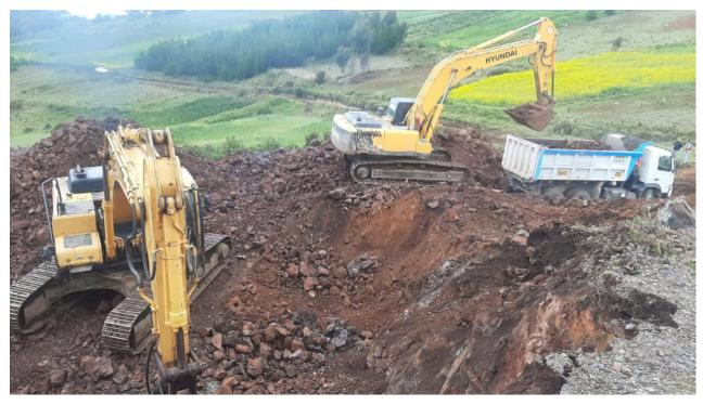
Figure 2. Loading of Ore onto trucks for delivery to crushing plant
