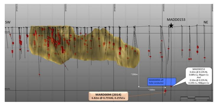
Figure 2: Long section of Maibele North resource (brown shape) plus extensional areas to the west and east.
