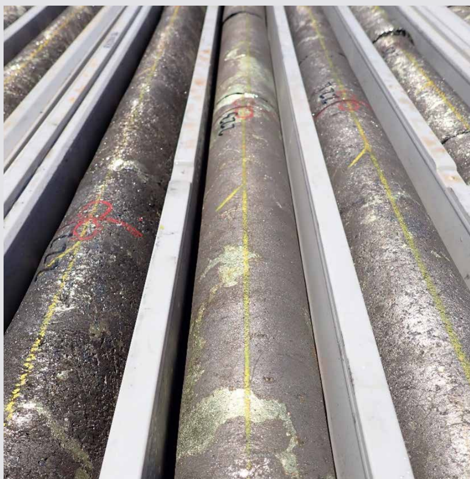
PHOTO 1 - MASSIVE Ni-Cu SULPHIDE WITH LOOP TEXTURE FROM RKDD034 FROM 223M, NQ2
