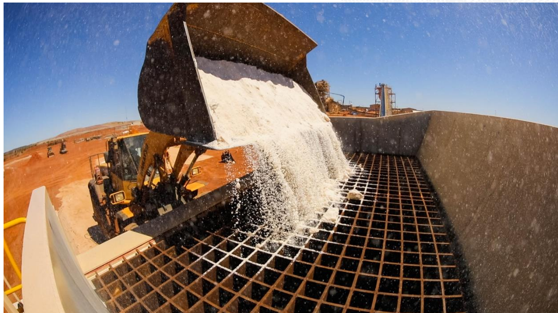
Figure 1: First bucket of salt fed into the feed hopper
