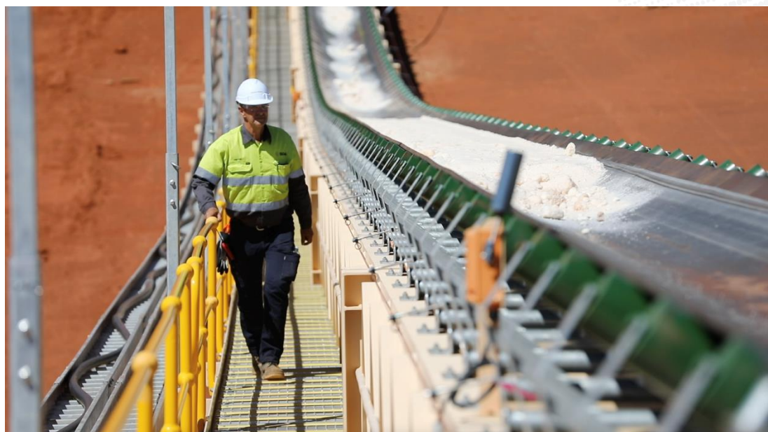
Figure 2: Conveyer CV01 operating with first feed salts
