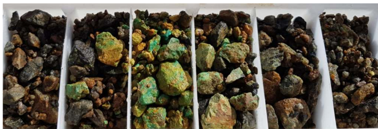
Image 13 | Nanadie Well RC Drilling Rock Chips: 8-13m NWRC21031
