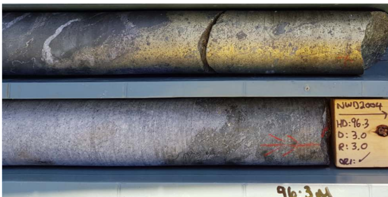
Image 8 | NWD2004 drill core 92.5m to 96.3m downhole showing chalcopyrite copper sulphide mineralisation
