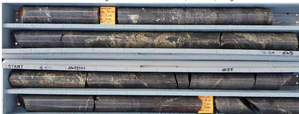
Image 9 | NWD2101 drill core 75.3m to 78.3m downhole showing chalcopyrite and pyrrhotite mineralisation
