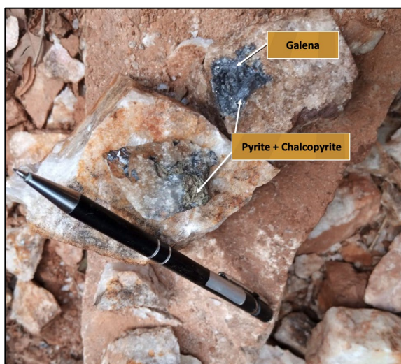
Figure 7 – Dragon Target: photo showing quartz veining with tourmaline-pyrite-chalcopyrite-galena mineralisation
