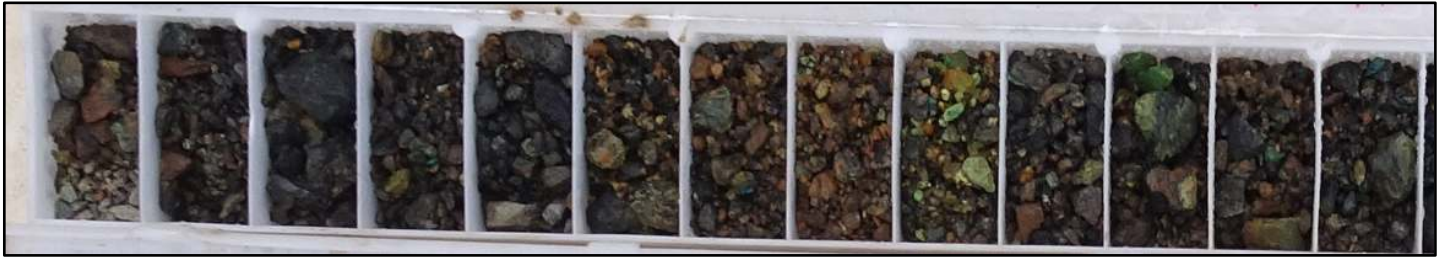
Image 1 | Nanadie Well RC Drilling Rock Chips: NWRC21006 from 20-33m (includes 9.0m at 1.6% Cu malachite mineralisation 20-29m)
