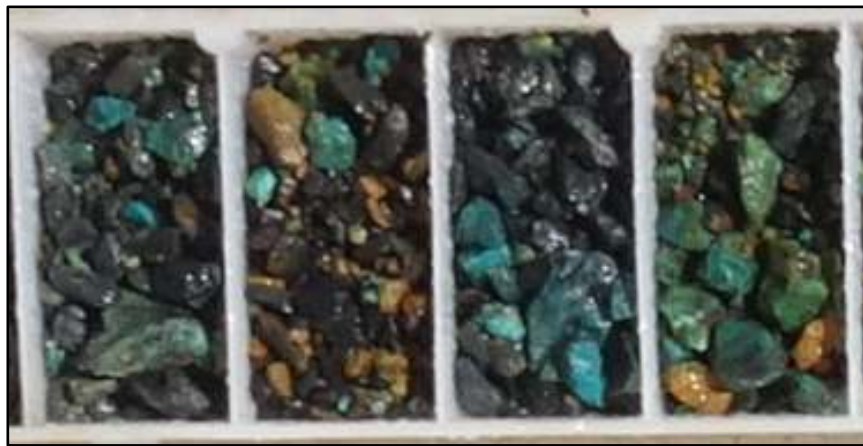
Image 2 | Nanadie Well RC Drilling Rock Chips: NWRC21011 from 25m-29m (4.0m at 2.4% Cu malachite/chrysocolla mineralisation)
