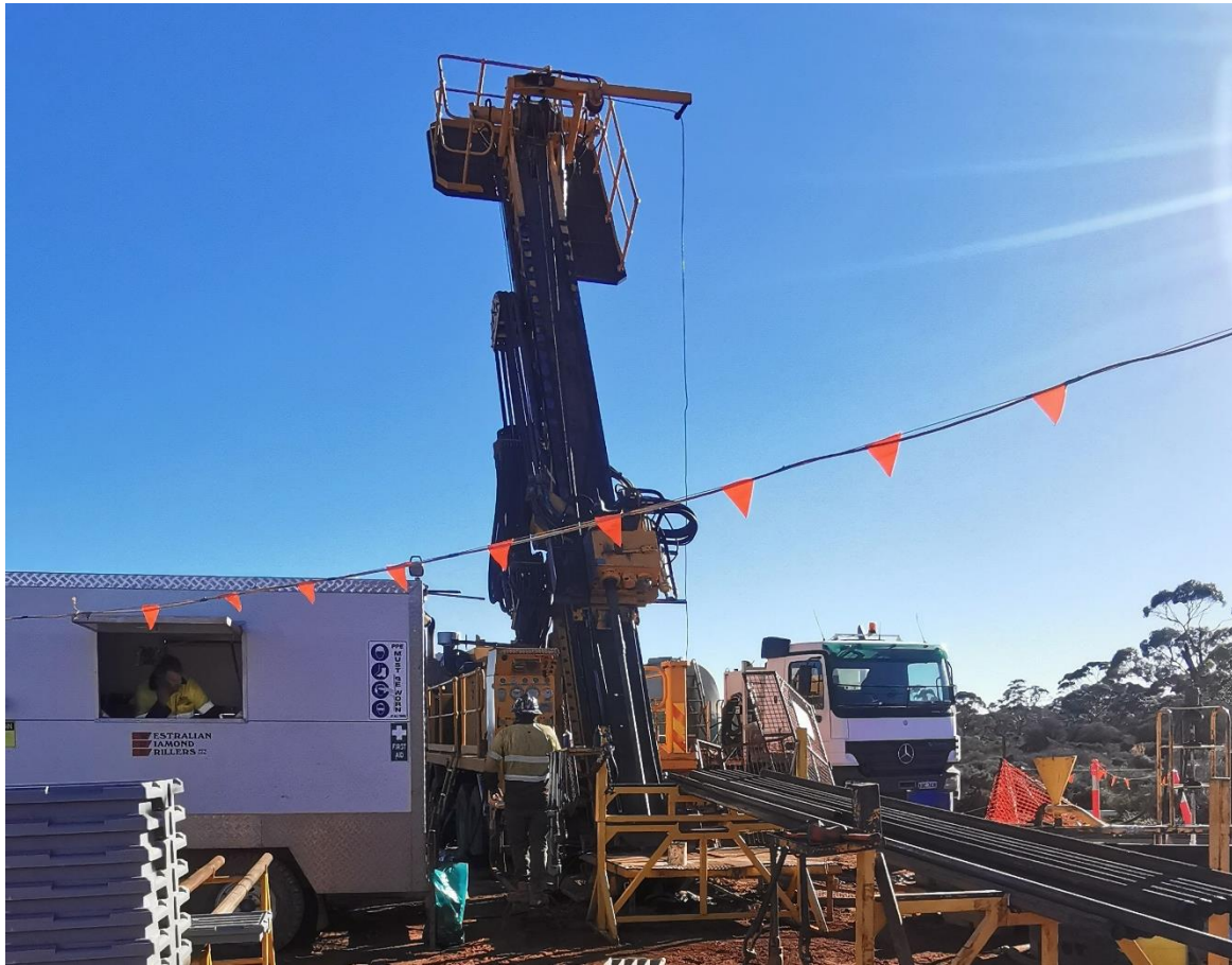
Image 2 – Diamond drilling in progress at Mandilla East
