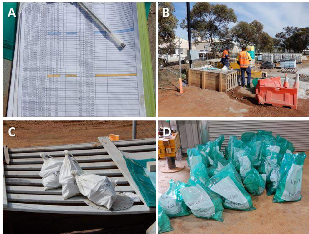
Figure 11-2: Drill core sampling. A: Cut sheet created by geologist. B: Cutting core on Almonte saw, Parkes facility. C: Pre-numbered sample bags. D: Bagged samples ready for zip-tying and dispatch to laboratory
