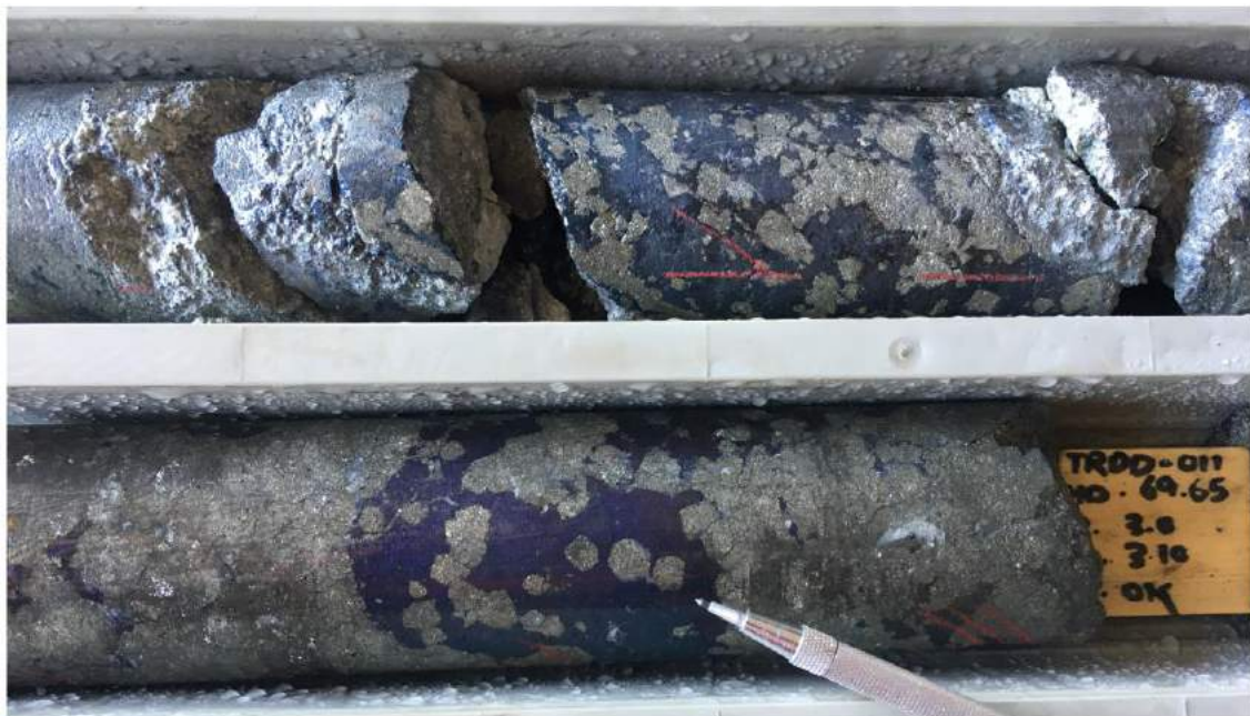
Figure 6-6: Massive sulphide skarn mineralisation, TRDD011. Coarse pyrite with blue-purple covellite and dark grey chalcocite, 68.5 m-69.65 m.
