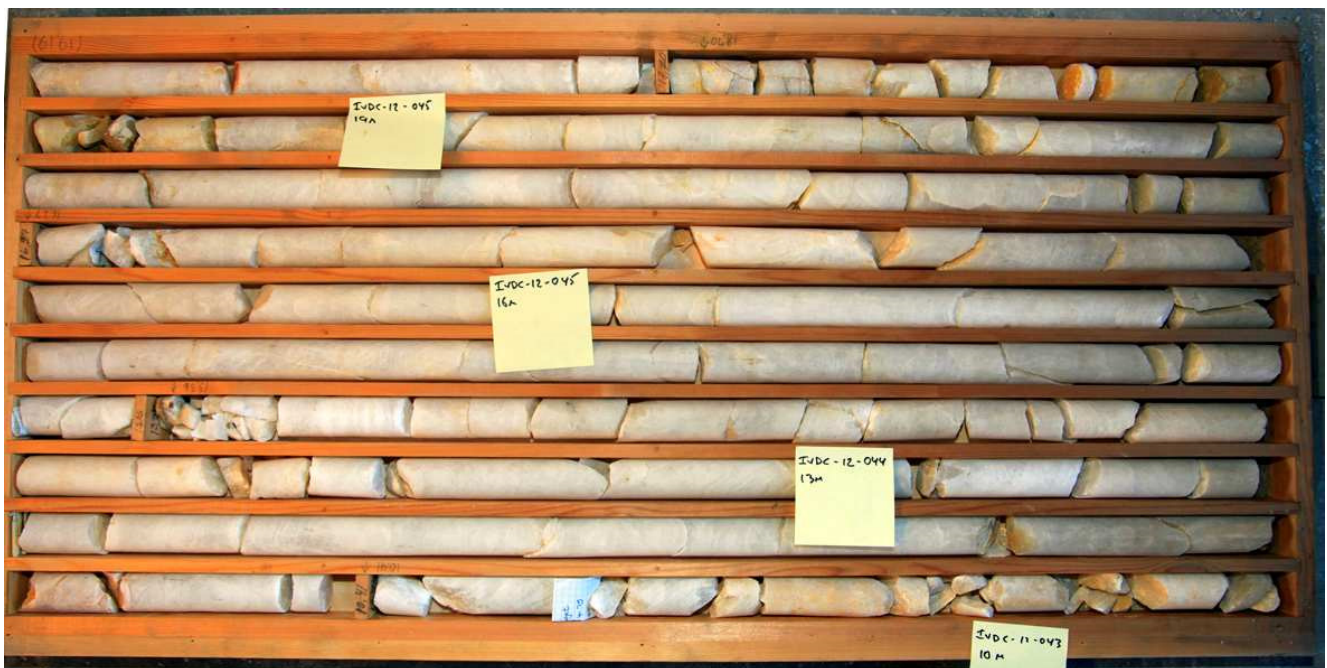
Figure 4: High silica grade quartz from Drill Hole 153
