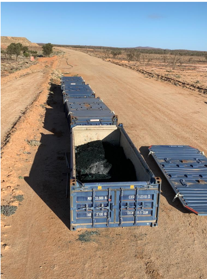
Figure 1: Containers at site being loaded with copper concentrate
