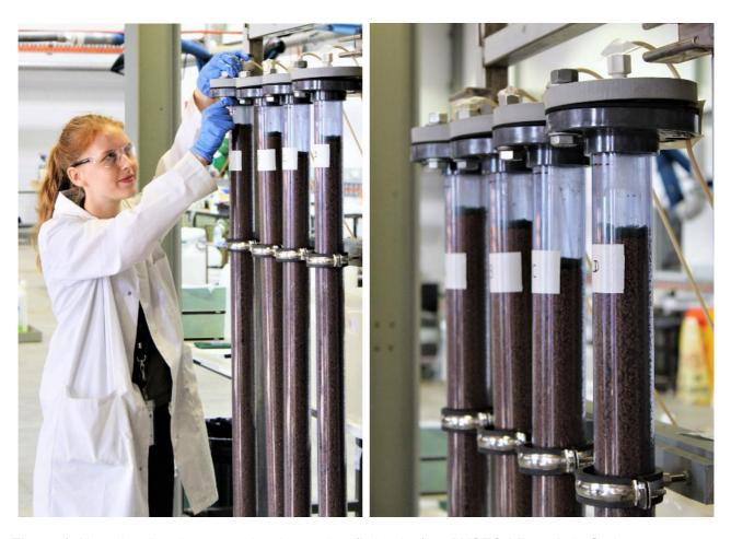
Figure 1: Heap leach columns under desorption (irrigation) at ANSTO Minerals in Sydney.
