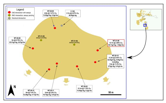
Figure 4 – Elevation view with mineralised intersections at the Leatherwood-sediments contact. The drill rig will continue infill drilling and test the southern extension of this lode after drill pad preparation is completed (Note that the mineralisation has an overall easterly dip at approximately 45°. The view above is perpendicular to the best plane approximating the mineralisation).
