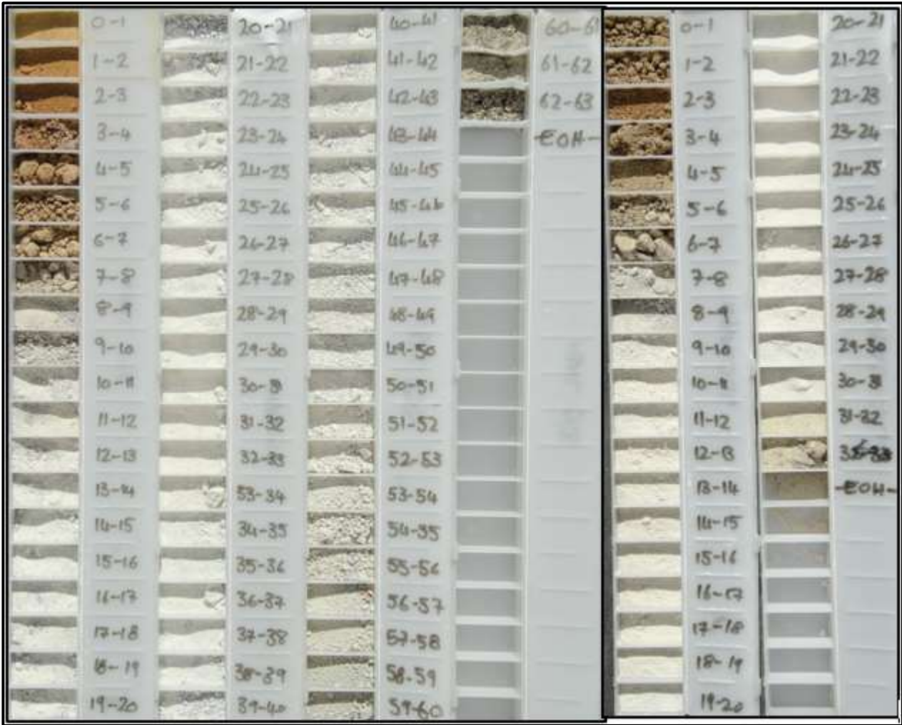
Figure 4 – Air-core drill cuttings from Drill holes 4 NBAC058 (0-63m) left, and NBAC044 (0-33m) right
