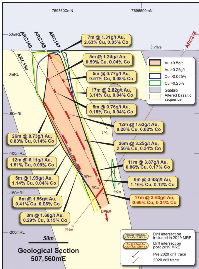
**Figure 4:** Cross-section view of the Carlow Castle Main Eastern Zone on section 507,560mE. Hole ARC276 has extended the high-grade shoot down dip a further 30m and being drilled normal to the dip direction
