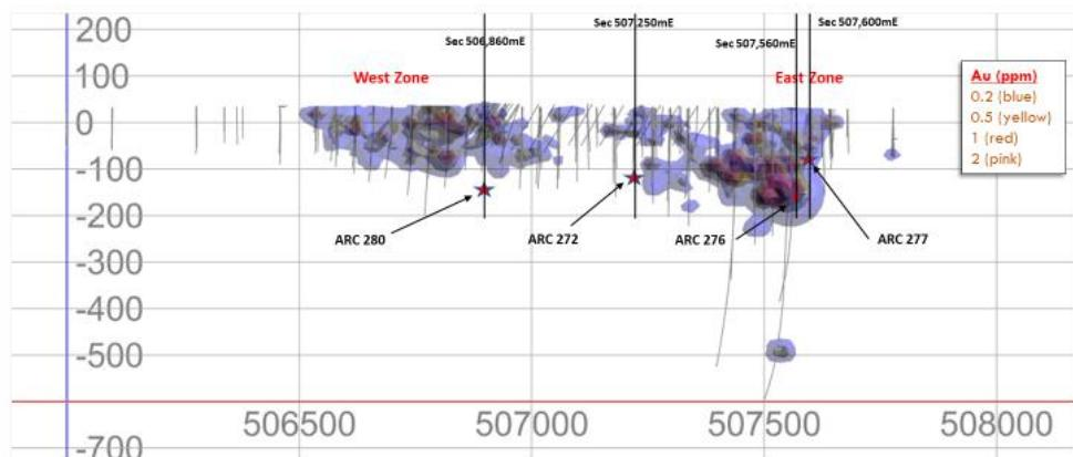
**Figure 2:** Carlow Castle Main Zone; 3D Isometric Leapfrog image of Au mineralization contours, looking north. Showing location of (RC) hole locations for ARC272, ARC276, ARC277, ARC280 on the Main Zone, east and west areas
