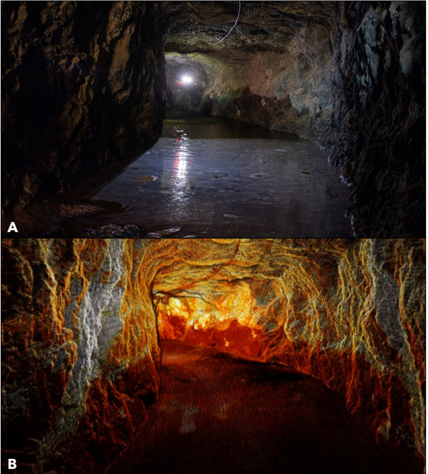
Figure 4; A – Hovermap® drone system mapping workings down to the water level using LiDAR. B - Resulting LiDAR digital image post processing.
