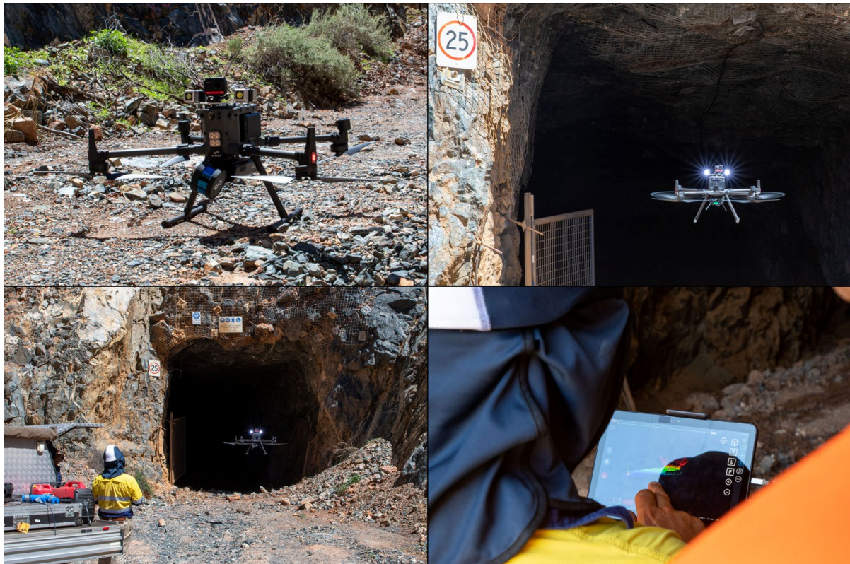
Figure 3; Sensorem Hovermap® drone system commencing LiDAR survey of the First Hit mine workings.
