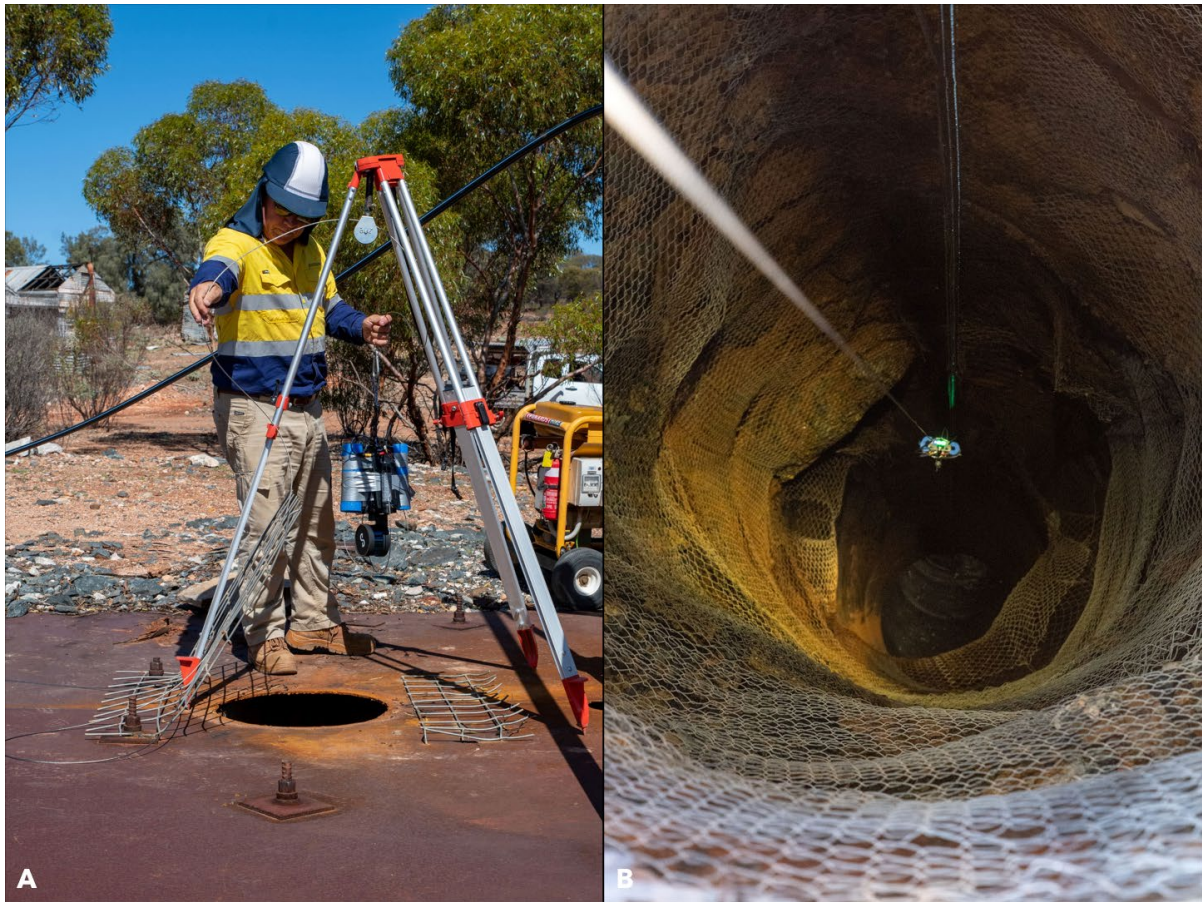
Figure 2; A - Sensorem undertaking a LiDAR survey of the vent raise connecting the underground workings to surface. B - LiDAR unit being lowered down in to the vent raise.
